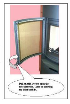
A torsion spring is used to automatically close this door. This spring should never be disabled (refer to DIN 18891, Type 1). The door <u>must</u> be locked manually.
